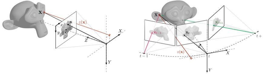
**Fig. 2. Left:** Illustration of the employed depth parametrization. **Right:** Illustration of corresponding points defined by the image location  $\mathbf{x}_t$  and the associated depth value  $z(\mathbf{x}_t)$ . In this case, the 3D point is occluded in one view and could be handled with the idea of temporal selection. i.e. by the view from the other time step.
