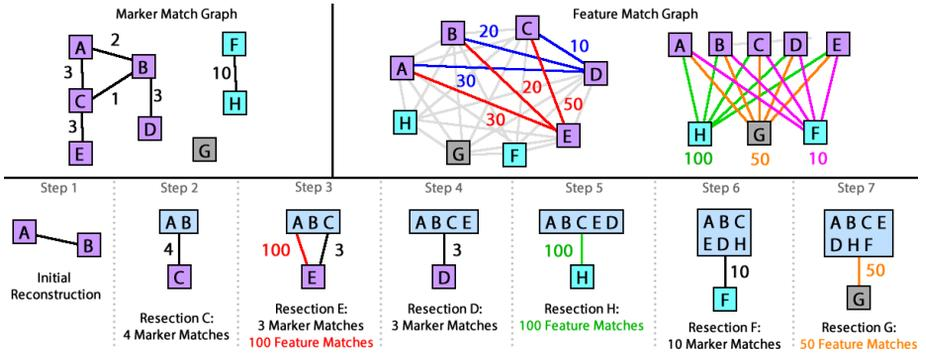
**Fig. 6.** The top left diagram depicts images as lettered boxes with edges representing the number of matched markers between image pairs. The top middle and top right diagrams depict the number of common feature matches between images. The bottom diagram depicts the resectioning order of images A to G based on two rules: (1) add the image that shares the most marker matches with the reconstruction; (2) break ties using most shared feature matches.
