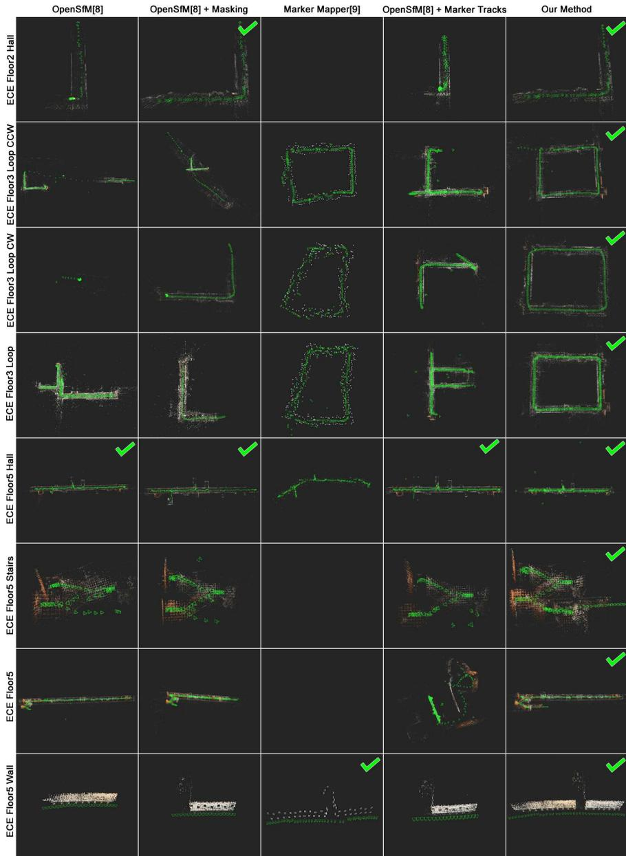
**Fig. 7.** Reconstructions for OpenSfM, OpenSfM with markers masked, MarkerMapper, OpenSfM with marker tracks, and our method on the ECE image collections. Using the markers as texture often produces worse results (e.g. *ECE Floor2 Hall*, *ECE Floor3 Loop CW*, *ECE Floor3 Loop*, and *ECE Floor5 Stairs*). Our method produces complete reconstructions that are as good or better than the other methods for all image collections. The best results are denoted by a green check mark.
