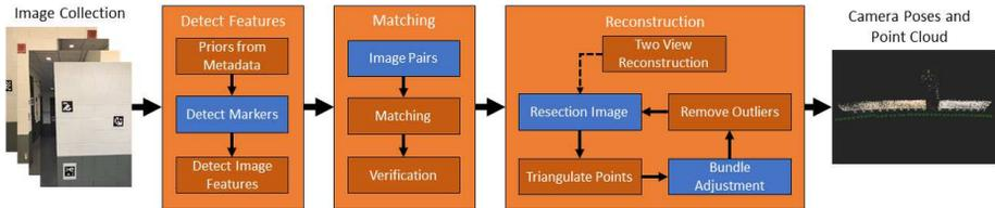
**Fig. 5.** This diagram depicts the typical incremental SfM approach: extracting priors from metadata (e.g. focal length), detecting features, matching features, and reconstruction. The blue boxes are the areas we added or changed in our method.
