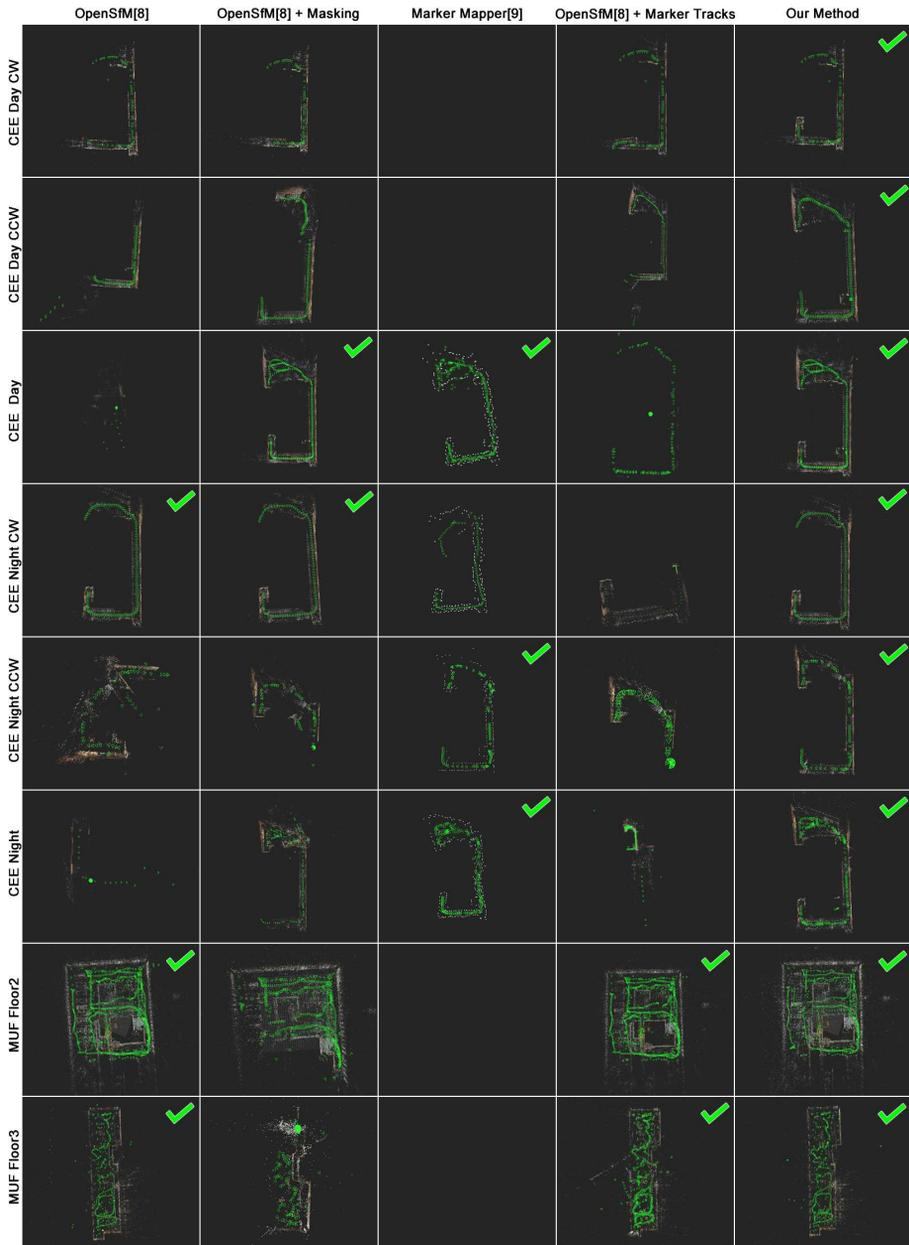
**Fig. 8.** Reconstructions for OpenSfM, OpenSfM with markers masked, MarkerMapper, OpenSfM with marker tracks, and our method on the CEE and MUF image collections. Again, using the markers as texture often produces worse results (e.g. *CEE Day CCW*, *CEE Day*, and *CEE Night*). Our method produces complete reconstructions that are as good or better than the other methods for all image collections. The best results are denoted by a green check mark.
