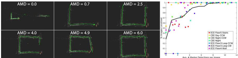
**Fig. 9.** The left six images show how the reconstruction of *ECE Floor3 Loop CCW* improves as marker density increases. Here AMD means average marker detections per image. The right image shows the percent of images localized as the AMD increases. Each color represents a different dataset. The trend line is shown in black. As the AMD increases, the percent of localized images increased to 100%.
