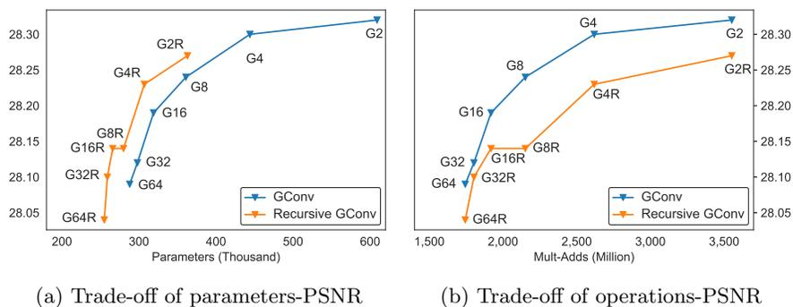
Fig. 5: Results of using efficient residual block and recursive network in terms of PSNR vs. parameters(**left**) and PSNR vs. operations(**right**). We evaluate all models on Set14 with  $\times 4$  scale. *GConv* represents the group size of group convolution and *R* means the model with the recursive network scheme (i.e., *G4R* represents group four with recursive cascading blocks).
