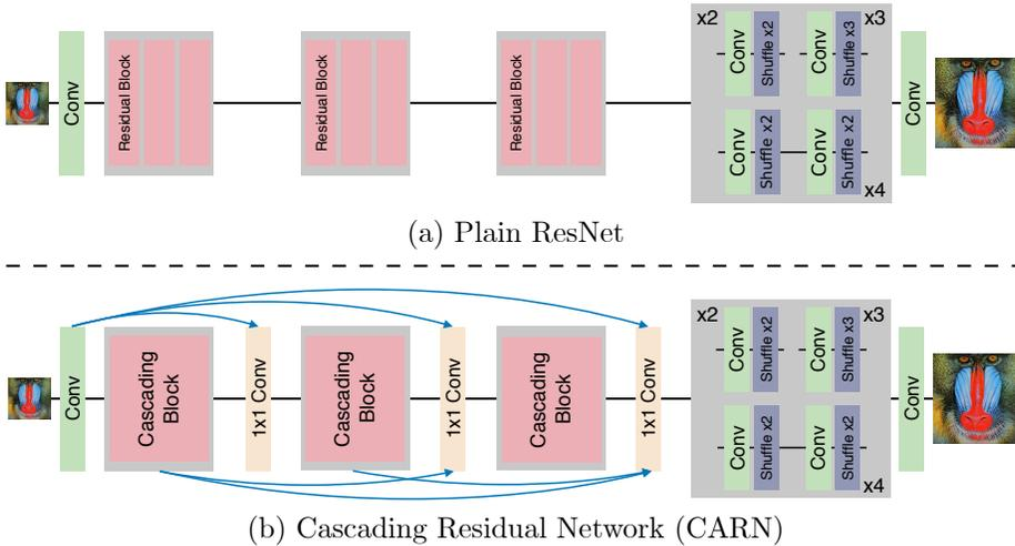
Fig. 2: Network architectures of plain ResNet (**top**) and the proposed CARN (**bottom**). Both models are given an LR image and upsample to HR at the end of the network. In the CARN model, each residual block is changed to a cascading block. The blue arrows indicate the global cascading connection.
