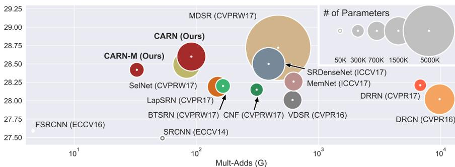
Fig. 4: Trade-off between performance vs. number of operations and parameters on Set14  $\times 4$  dataset. The  $x$ -axis and the  $y$ -axis denote the Multi-Adds and PSNR, and the size of the circle represents the number of parameters. The Multi-Adds is computed by assuming that the resolution of HR image is 720p.
