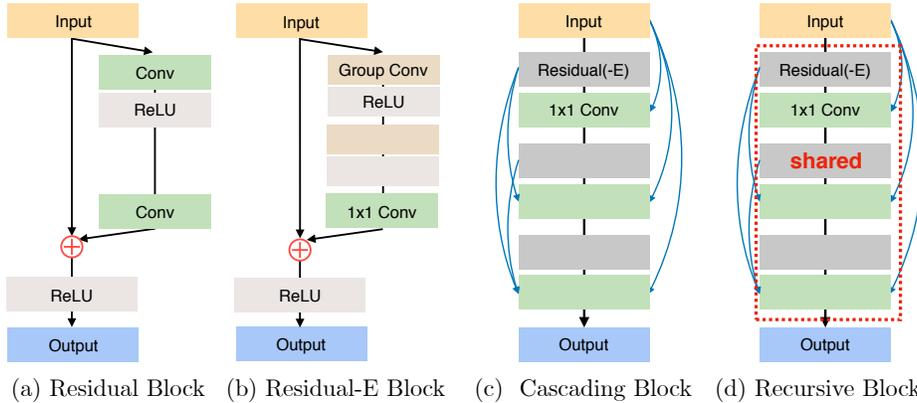
Fig. 3: Simplified structures of (a) residual block (b) efficient residual block (residual-E), (c) cascading block and (d) recursive cascading block. The  $\oplus$  operations in (a) and (b) are element-wise addition for residual learning.
