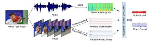
**Fig. 4.** Testing pipeline. Given a novel test video, we detect the objects present in the visual frames, and retrieve their learnt audio bases. The bases are collected to form a fixed basis dictionary **W** with which to guide NMF factorization of the test video's audio channel. The basis vectors and the learned activation scores from NMF are finally used to separate the sound for each detected object, respectively.
