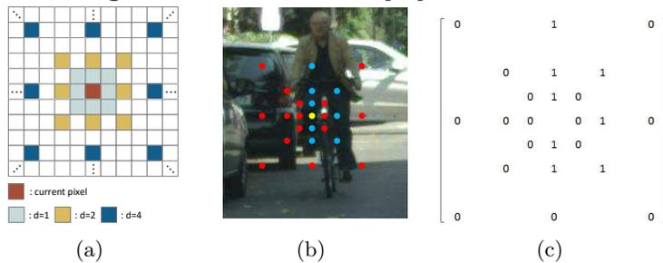
**Fig. 2.** Illustration for pixel affinity. (a) Locations for proposed neighbors. (b) The yellow point indicates the current pixel. Other points are neighboring pixels, in which red ones indicate pixels of different instances and blue ones indicate the same instance (*rider*). The pixel distance is NOT real but only for an illustration. (c) The derived labels and expected network output.
