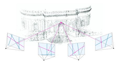
**Fig. 1: Privacy Preserving SfM.** Our proposed method takes privacy preserving feature lines as input and seeds the reconstruction from four views with at least eight corresponding line features. The intersection of at least three line features produces a point triangulation. Camera resectioning requiring at least six 2D line to 3D point correspondences is based on Speciale *et al.* [42].
