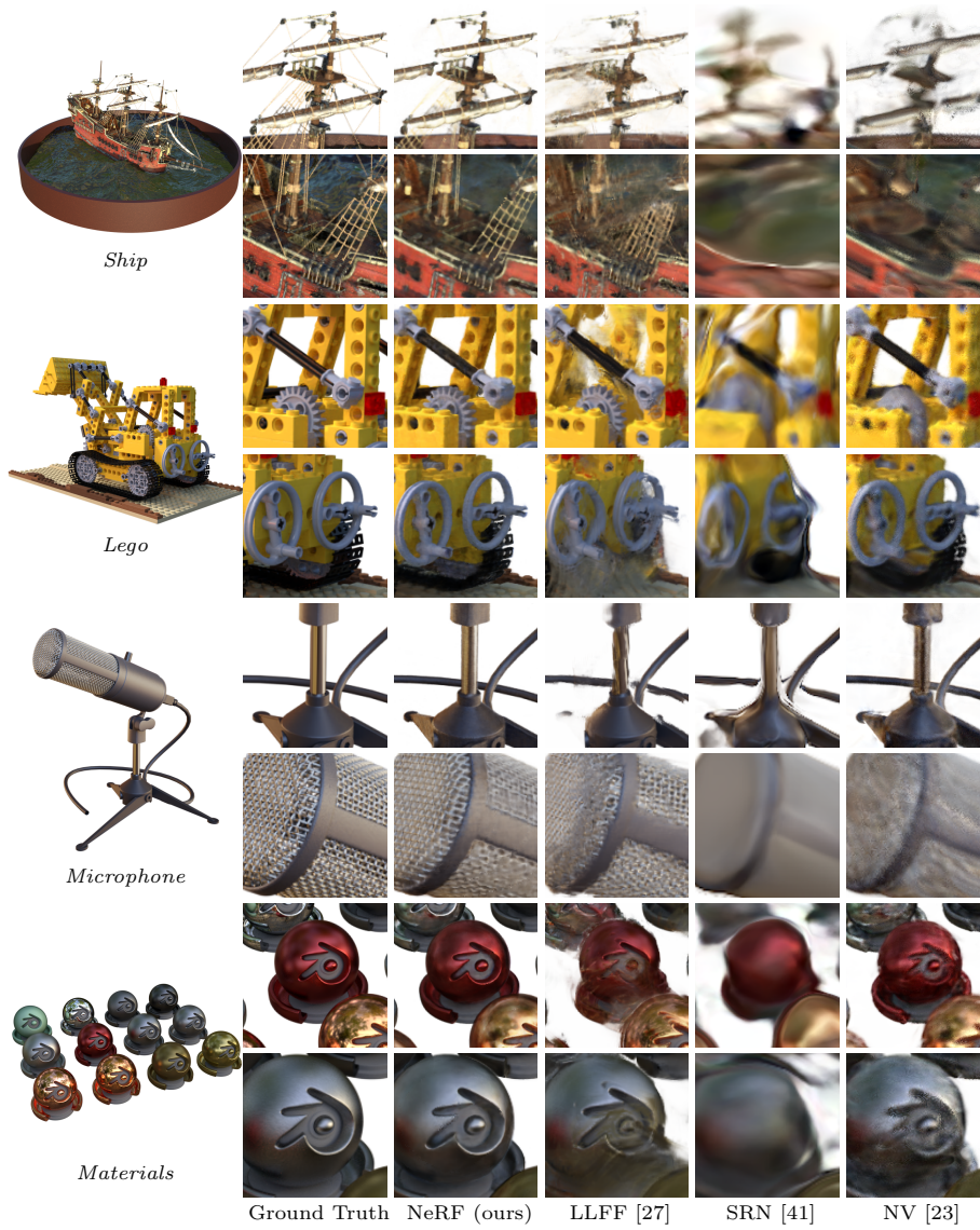
Fig. 5: Comparisons on test-set views for scenes from our new synthetic dataset generated with a physically-based renderer. Our method is able to recover fine details in both geometry and appearance, such as Ship ’s rigging, Lego ’s gear and treads, Microphone ’s shiny stand and mesh grille, and Material ’s non-Lambertian reflectance. LLFF exhibits banding artifacts on the Microphone stand and Material ’s object edges and ghosting artifacts in Ship ’s mast and inside the Lego object. SRN produces blurry and distorted renderings in every case. Neural Volumes cannot capture the details on the Microphone ’s grille or Lego ’s gears, and it completely fails to recover the geometry of Ship ’s rigging.
