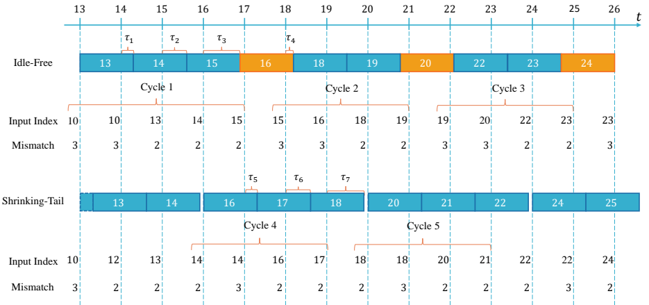
Fig. D. Shrinking-tail cycle (for 1 < r < 1.5 ). Intuitively, blocks within each shrinking-tail cycle has tails increasing ( \tau_1 < \tau_2 < \tau_3 and \tau_5 < \tau_6 < \tau_7 ). It ends when tail decreases or there is an idle gap, and thus the tail “shrinks”.
