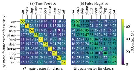
**Fig. 6.** The cosine similarity between mean feature vectors for a class (y-axis) and a row in the CSG matrix (x-axis), calculated on all TP/FN samples. We reorder classes in CIFAR10 for better visualization.
