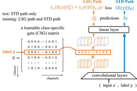
**Fig. 3.** In Class-Specific Gate (CSG) training, we *alternately* train a CNN through the CSG path and the standard (STD) path. In the CSG path, activations after the penultimate layer (i.e. the last convolution) pass through learnable gates indexed by the label. In training, network parameters and the gates are optimized to minimize the cross-entropy joint with a sparsity regularization for the CSG matrix. In testing, we just run the STD path.
