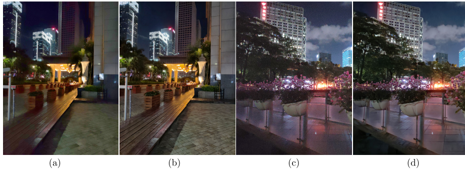
Fig. 1: Our proposed denoising method can run smoothly on smartphones with high quality noise reduction even in low-light conditions (see (b),(d)). In contrast, the default ISP image denoiser produces images with over-smoothed high texture regions (e.g. ground in (a)) and noisy smooth regions (e.g. sky in (c)).
