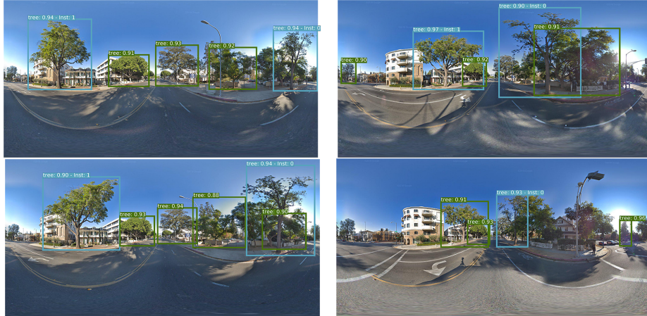
Fig. 3. Sample results obtained on the Pasadena dataset for multi-view object detection and re-identification. Trees were correctly detected (green) and further accurately re-identified across different views (cyan) when possible.
