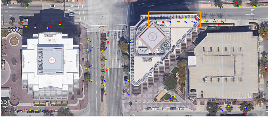
Fig. 5. Sample of geo-localization results for Pasadena comparing different methods. Green, blue, yellow and red circles represent the ground-truth, GeoGraph, SSD-ReID-Geo and MRF respectively. The orange bounding box exhibits how ground level imagery can be helpful to detect object obscured by buildings from aerial view.
