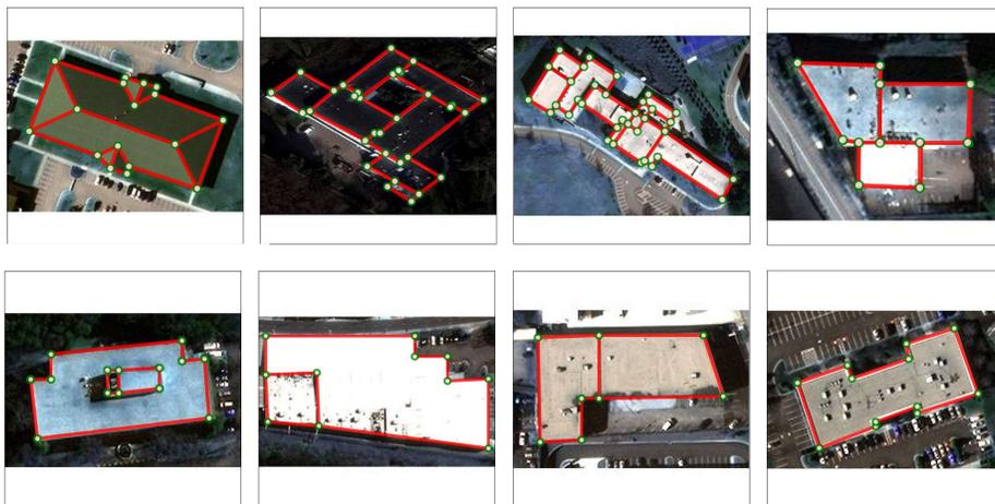
**Fig. 2.** Sample input RGB images and their corresponding planar graph annotations.
