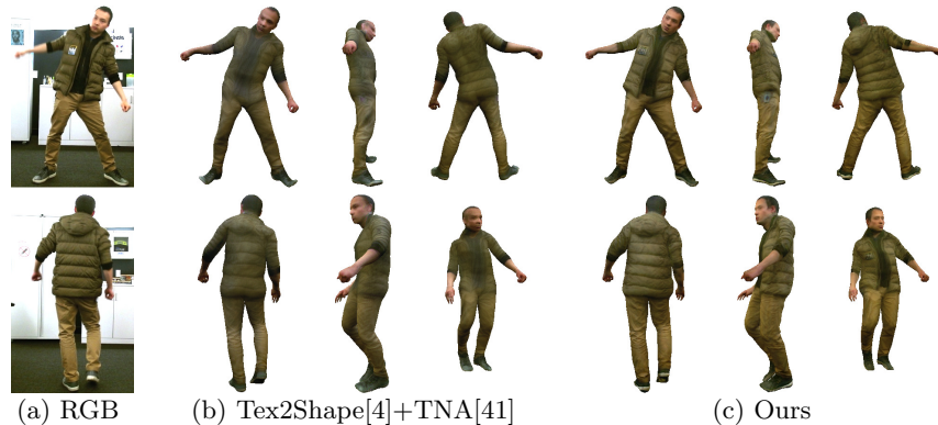
Fig. 1. Tex2Shape [4] + TNA [41] vs. Our Result. The mesh with texture is rendered from different viewpoints. Our approach reconstructs more detailed geometry, such as the moving jacket, as well as more accurate texture.
