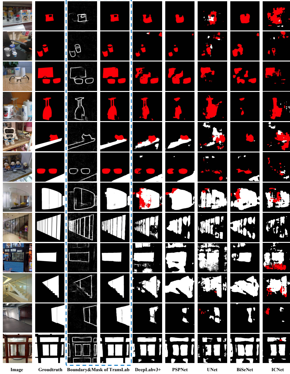
Fig. 5. More visual comparison of TransLab to other semantic segmentation methods. Our TransLab clearly outperforms others thanks to the boundary attention.
