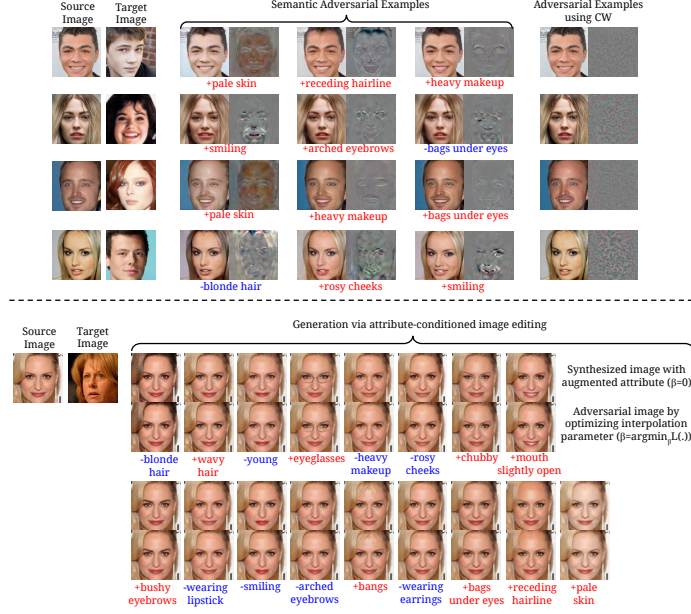
Fig. 3. Top: Qualitative comparisons between our proposed SemanticAdv and pixel-wise adversarial examples generated by CW [12]. Along with the adversarial examples, we also provide the corresponding perturbations (residual) on the right. Perturbations generated by our SemanticAdv (G-FPR = 10^{-3} ) are unrestricted with semantically meaningful patterns. Bottom: Qualitative analysis on single-attribute adversarial attack (G-FPR = 10^{-3} ). More results are shown in the supplementary
