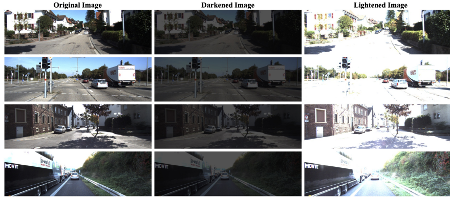
Fig. 4. Visualization of the darkened images and lightened images generated by the illumination transformation to simulate the underexposure and overexposure cases in the real scenes.
