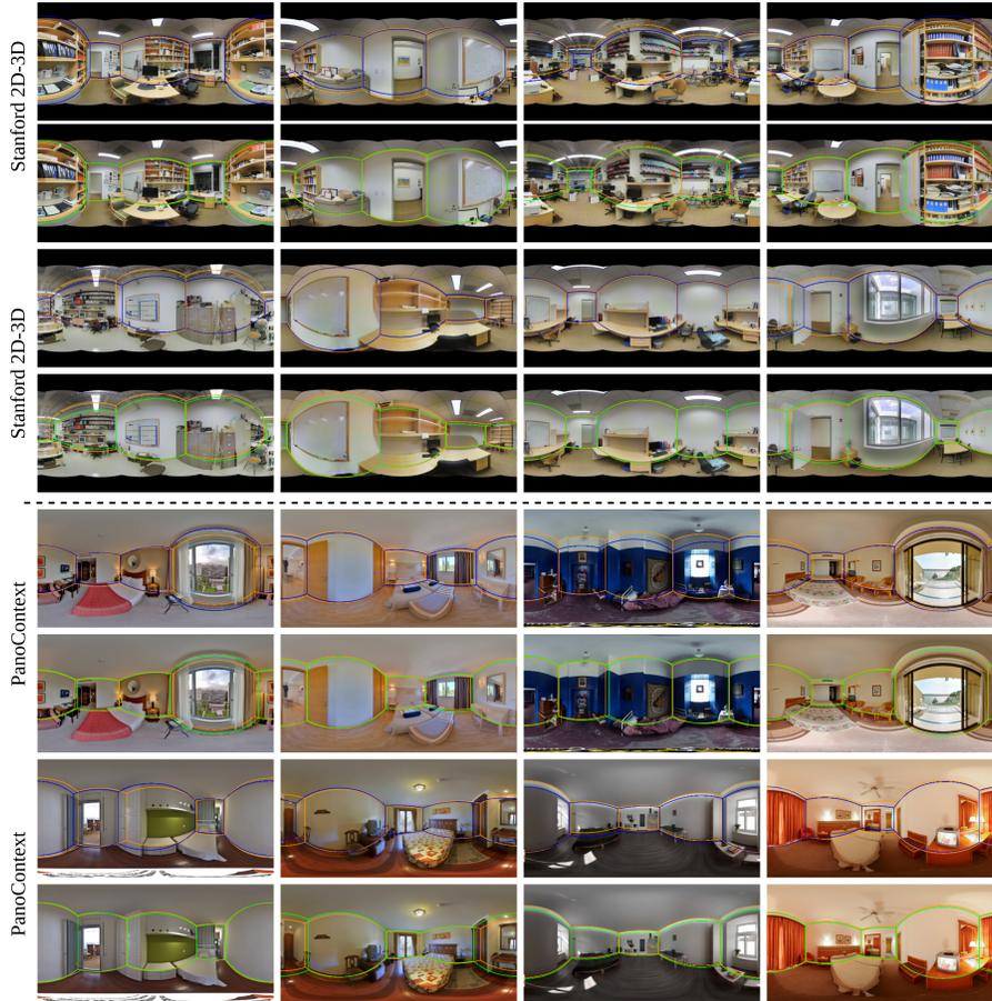
**Fig. 3.** Additional qualitative results on layout prediction. Results are shown of testing the baseline LayoutNet [5] and our proposed method on the Stanford 2D-3D dataset (top four rows) and PanoContext dataset (bottom four rows). For each example, we show the predicted layout (LayoutNet: blue, the proposed method: green) and the ground truth (orange) under equirectangular view
