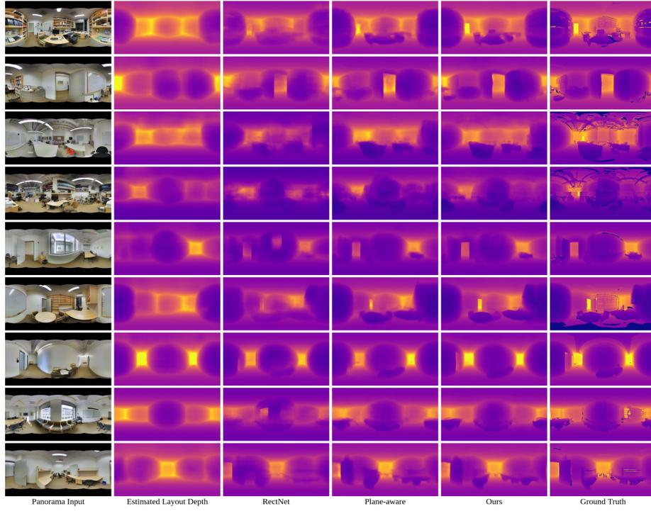
**Fig. 6.** Additional qualitative results on depth estimation. Results are shown for experiments of testing the estimated layout depth map, the baseline RectNet [4], Plane-aware network [1] and our proposed method on the Stanford 2D-3D dataset
