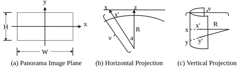
**Fig. 1.** Geometry derivation for equirectangular reprojecting layout depth map from 3D layout points
