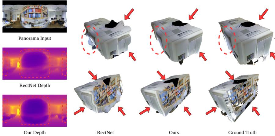
**Fig. 7.** Additional 3D reconstruction comparison. Due to the explicitly inter-positioning of the layout depth, the proposed method predicts a relatively good depth map for the distant regions. So the 3D reconstruction of the proposed method is more proper and provides more planar ceiling and walls
