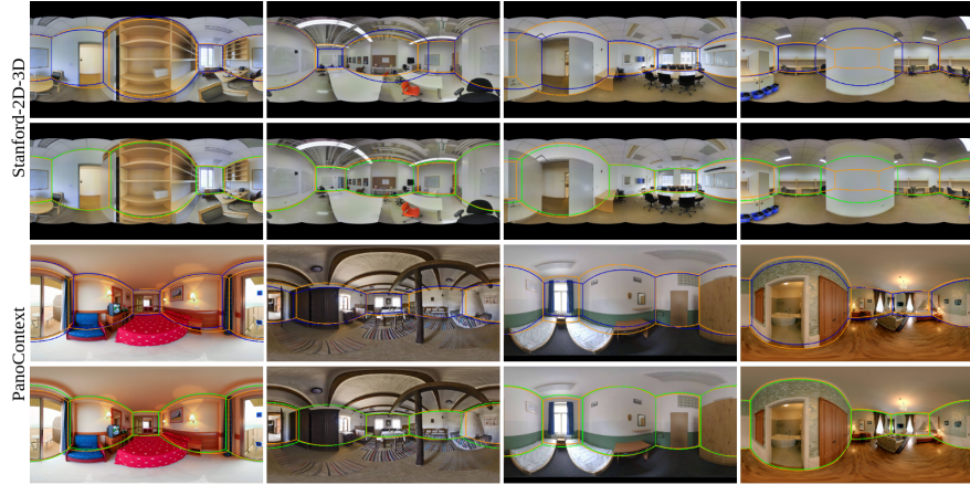
Fig. 4: Qualitative comparison on layout prediction. Results are shown of testing the baseline LayoutNet [35] (blue), our proposed method (green) and the ground truth (orange) on the Stanford 2D-3D dataset and PanoContext dataset
