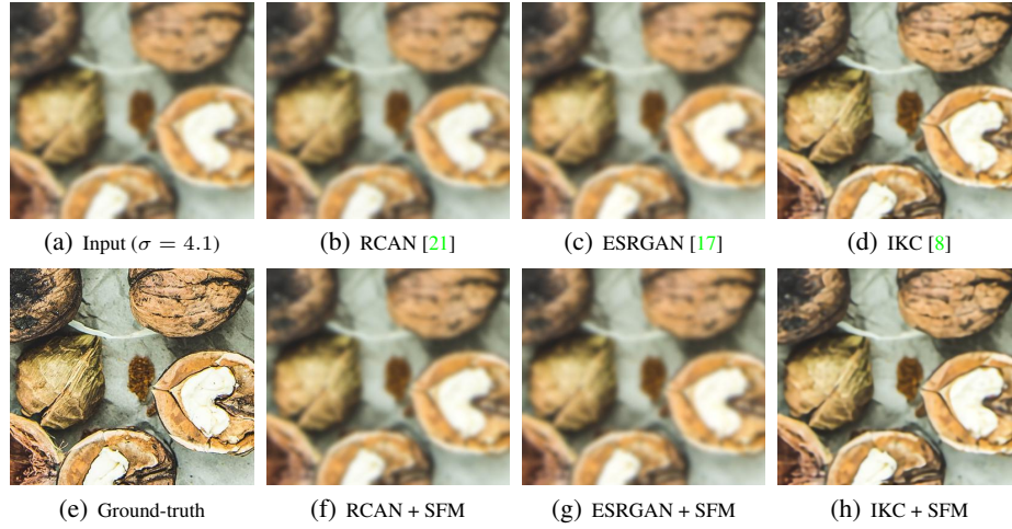
Fig. 5: Cropped SR results (x4 upscaling) with different methods (top row), and with the same methods trained with our SFM (bottom row), for image 0872 of the DIV2K benchmark.
