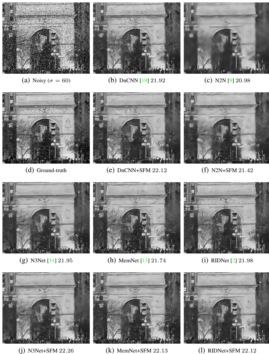
Fig. 13: Denoising results with different methods (1st and 3rd row), and with the same method trained with our SFM (2nd and 4th row), for image 21 of the BSD68 benchmark. We also show the PSNR values of every denoised result (in dB ).
