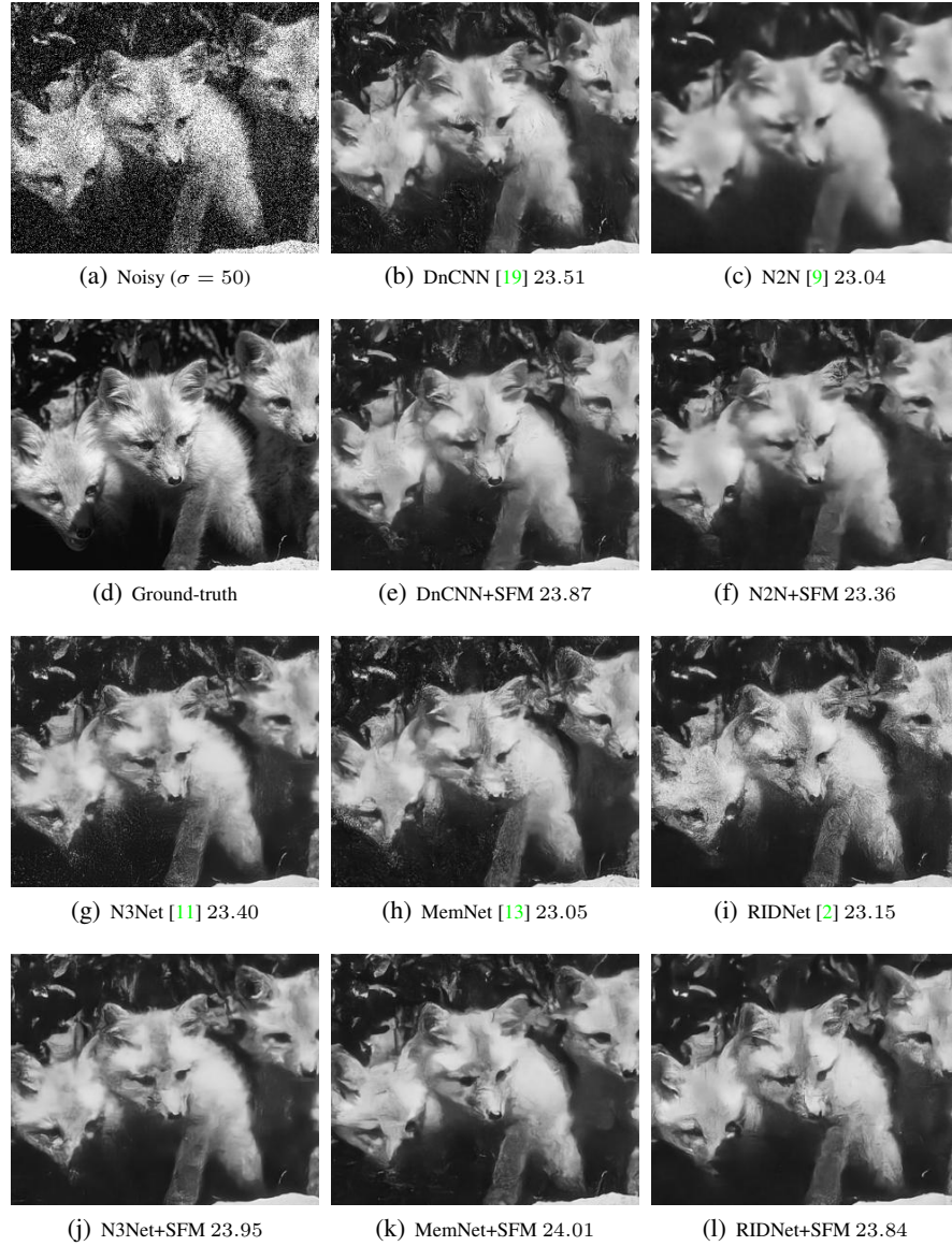
Fig. 14: Denoising results with different methods (1st and 3rd row), and with the same method trained with our SFM (2nd and 4th row), for image 23 of the BSD68 benchmark. We also show the PSNR values of every denoised result (in dB ).
