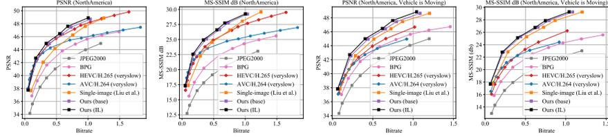
Fig. 7: Plot of our approaches compared against compression baselines for NorthAmerica, both over the entire dataset as well as only when the ego-vehicle has positive velocity.
