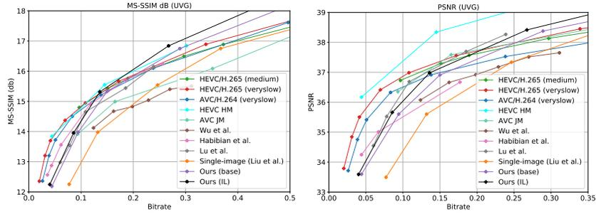
Fig. 5: Rate-distortion plot of our model against competing deep compression works [39, 14, 20]. Results are on full  $1920 \times 1080$  UVG video.
