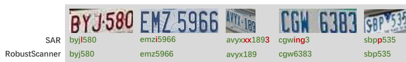
Fig. 5. Samples of recognition results of our RobustScanner and SAR [25] on the license plate dataset.
