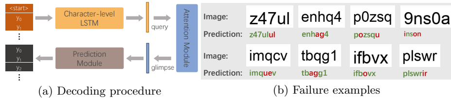
Fig. 1. Illustration of the decoding procedure of encoder-decoder with attention framework and its failure cases.
