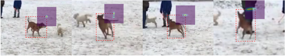
Fig. S2: Visualization of the conditional target density p(y|x;\theta) \propto e^{f_\theta(x,y)} predicted by our network for the task of bounding box estimation in visual tracking. Since the target space y \in \mathbb{R}^4 is 4-dimensional, we visualize the density for different locations of the top-right corner as a heatmap, while the bottom-left is kept fixed at the tracker output (red box). Our network predicts flexible densities which qualitatively capture meaningful uncertainty in challenging cases.
