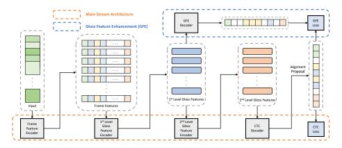
Fig. 1. Overview of the proposed network. The network is fully convolutional and divides the feature encoding process into two main steps. A GFE module is introduced to enhance the feature learning
