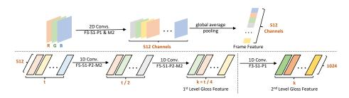
Fig. 3. The setting of the proposed main stream network. F, M refer to the filter size of convolution and max-pooling, respectively. S, P refer to the stride and padding size of convolution, respectively. Numbers aside are their actual size
