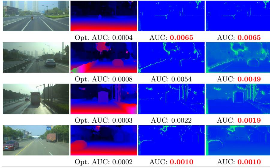
**Fig. 6. Online self-adaptation on DrivingStereo, GANet.** We extract 4 frames from the sequences selected for our experiments, respectively starting from first (top) and sampling every 2000 frames. For each frame, we show from left to right the reference image, disparity map using GANet and confidence maps estimated by OTB and OTB enabling self-adaptation.
