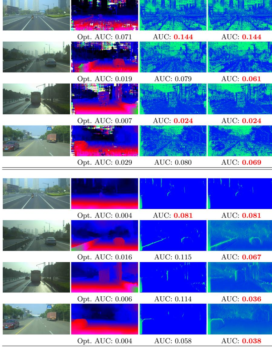
**Fig. 5. Online self-adaptation on DrivingStereo.** We extract 4 frames from the sequences selected for our experiments, respectively starting from first (top) and sampling every 2000 frames. For each frame, we show from left to right the reference image, disparity map using Census-SGM (top) or MADNet (bottom) and confidence maps estimated by OTB and OTB enabling self-adaptation.
