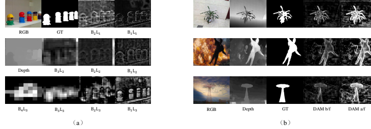
Fig. 6. (a) The visualization of the feature maps in FLM. The B_i L_j presents the output features of corresponding block in Fig. 2. (b) Visualization of the effectiveness of the DAM. The 4 th (DAM b/f) and the 5 th columns (DAM a/f) show the feature maps before and after adopting DAM, respectively
