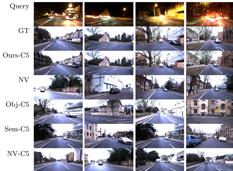
Fig. 6: Qualitative Results: For night time query images (top row), Ground Truth (GT) match (second row) and matches obtained from different methods are displayed (subsequent rows) including successful matches using our proposed representation (third row)
