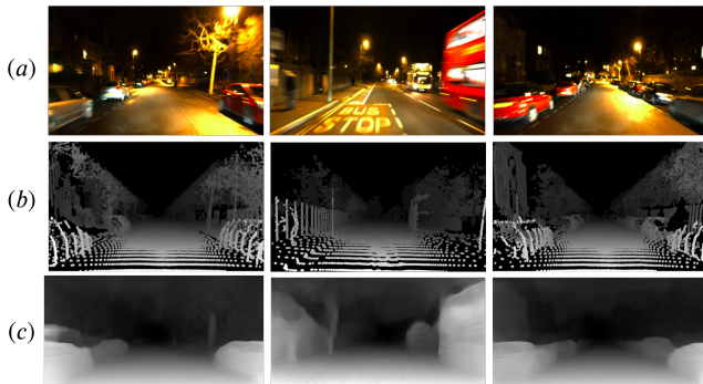
Fig. 1: The depth predictions of the proposed method on Oxford Night driving images. Top to bottom: (a) Input RGB night-time image. (b) Corresponding ground truth depth map generated from the LIDAR points. (c) The depth predictions using the proposed method
