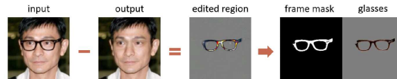
Fig. 7. Extracting eyeglasses from the glasses-removed images. These extracted eyeglasses can be used for synthesizing training pairs.
