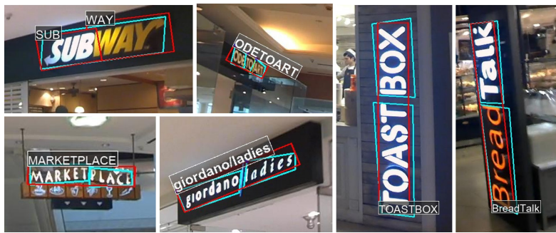
Fig. 9. Failure cases in IC15 dataset due to granularity difference. Red boxes denote detection results, cyan boxes denote ground truths.
