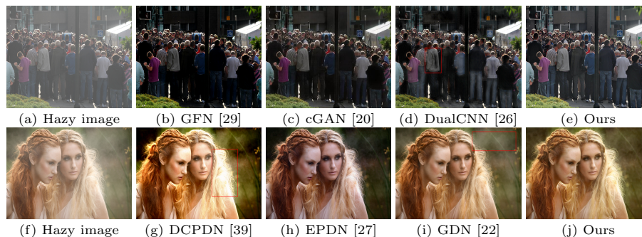
Fig. 4. Image dehazing results on real examples. The colors of the dehazed images in (b), (c), and (h) look darker. The part enclosed in the red box of (d) contains significant artifacts, e.g., the coat. The result in (g) has severe color distortions as shown in the red box. The image in (i) still contains some haze residuals. The proposed approach generates much clearer images (best viewed on high-resolution display with zoom-in).
