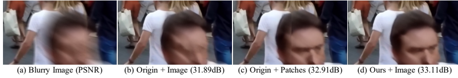
Fig. 2: Visual comparison with different test-time methods to MPRNet [56] for image deblurring. (a) Blurry image; (b) Inference with image; (c) Inference with cropped patches; (d) Ours: TLC is adopted and inference based on images. Our TLC generates sharp image without boundary artifacts in (b).
