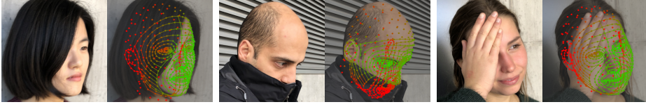
Fig. 5. When parts of the face are occluded by e.g. hair or clothing, the corresponding landmarks are predicted with high uncertainty (red), compared to those visible (green).
