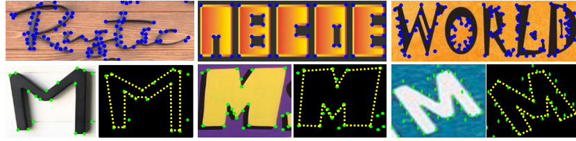
Fig. 3. Visualization of corner point detection. Top: The detected corner points of artistic text images. Bottom: Corner points of a character “M” with various appearances, whose structural relations are similar
