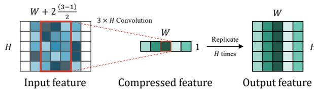
Fig. 4: Illustration of the proposed  $3 \times H$  WSM layer.
