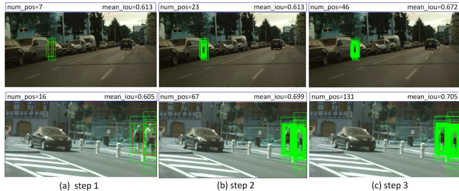
Fig. 2. Two examples from the CityPersons [44] training data. Green and red rectangles are anchor boxes and groundtruth boxes, respectively. Values on the upper left of the image represent the number of anchor boxes matched with the groundtruth under the IoU threshold of 0.5, and values on the upper right of the image denote the mean value of overlaps with the groundtruth from all matched anchor boxes.
