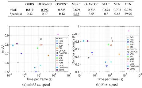
Fig. 4: **Performance comparison on the DAVIS-16 validation set.** The x axis denotes the average running time per frame in seconds (log scale) and the y axis is (a) mIoU (Jaccard index) and (b) F score (contour accuracy).
