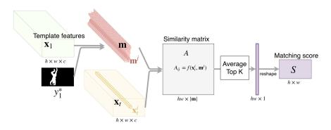
Fig. 2: **Illustration of the proposed soft matching layer.** We first take two sets of features and compute pairwise similarity between all pairs of features. We then produce the final matching score by computing the average of top K similarity scores.
