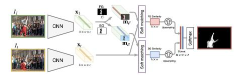
Fig. 1: Overview of the proposed video object segmentation algorithm. We use the provided ground truth mask of the first frame to obtain the set of foreground and background features ( $\mathbf{m}_F$  and  $\mathbf{m}_B$ ). After extracting the feature tensor  $\mathbf{x}_t$  from the current frame, we use the proposed soft matching layer to produce FG and BG similarity. We then cancatenate the two similarity scores and generate the final prediction via softmax.
