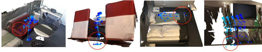
Fig. 8: Visualization of failure cases. In each red circle area, we observe the intersection between the human feet and the 3D mesh, e.g., the bed.
