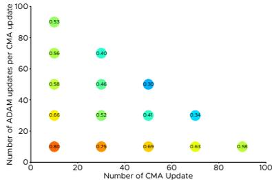
Fig. 15. **BasinCMA update ablation:** We plot the VGG L-PIPS score when we vary the number of CMA updates (x-axis) and the number of ADAM updates (y-axis). Lower is better.
