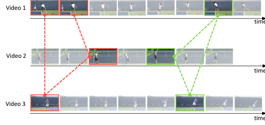
Fig. 3: An illustration of cycle consistency. The green lines denote a set of consistent correspondences and the red lines show a set of inconsistent correspondences.
