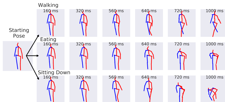
Fig. 4: Starting from a neutral pose, the grammar is able to generate multiple sequences by selecting different rules. Top: a walking sequence, middle: eating, bottom: sitting.
