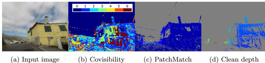
Fig. 5: Initial depth as obtained by multi-view stereo using PatchMatch (c) may contain spurious values. We clean the estimated depth by checking for consistency across several neighboring images (b). Only the depth values that are consistent with at least 3 neighbors are kept (d)
