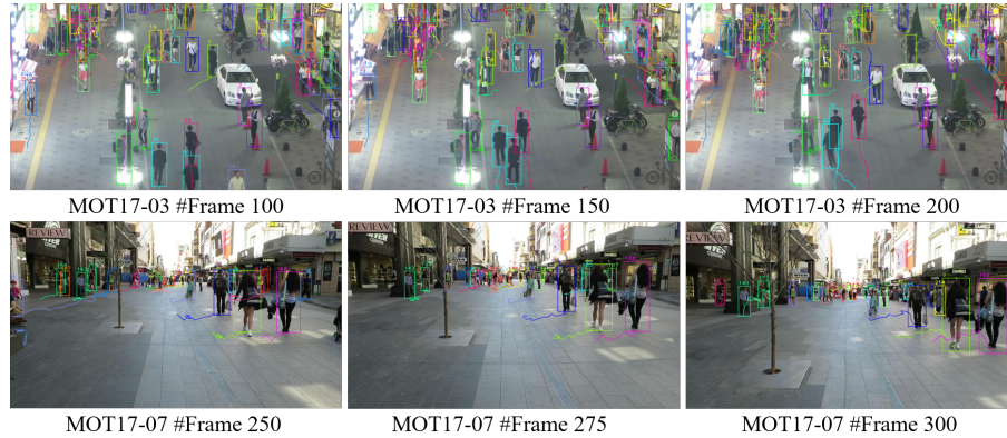
Fig. 5. Qualitative results of our CTracker on MOT17 test dataset. MOT17-03 sequence is captured by a static camera and MOT17-07 sequence is captured by a moving camera. The detected bounding boxes and the tracking trajectory with the same identity are displayed by the same color.
