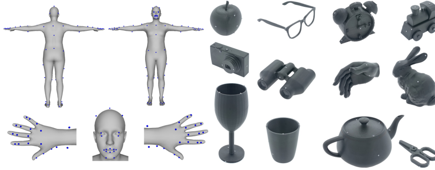
Fig. 2: MoCap markers used to capture humans and objects. Left: We attach 99 reflective markers per subject; 49 for the body, 14 for the face and 36 for the fingers. We use spherical 4.5 mm radius markers for the body and hemi-spherical 1.5 mm radius ones for the hands and face. Right: Example 3D printed objects from [5]. We glue 1.5 mm radius hemi-spherical markers (the gray dots) on the objects. These markers are small enough to be unobtrusive. The 6 objects on the right are mostly used by one or more hands, while the 6 on the left involve “whole-body grasps”.
