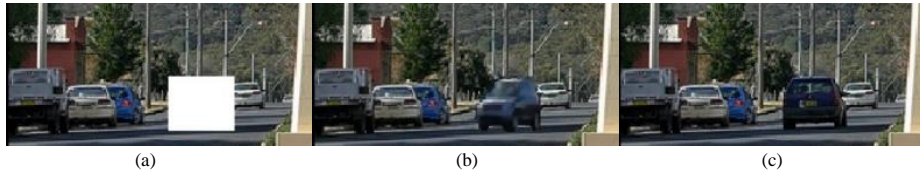
Fig. 7: An example that our method produces visually and structurally reasonable, yet distorted image completion, in this case the distorted car. Image (a) (b) and (c) respectively denote the input, our restoration image, and the ground truth.
