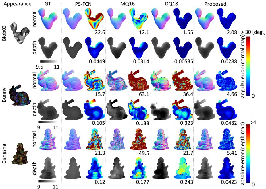
**Fig. 3.** Estimated results for our synthetic dataset. For each scene and each method, we show the estimated surface normal map, the depth map, the normal error map, and the depth error map. “GT” shows the ground truth of normals and depth. The numbers underneath the error maps show mean angular error in degrees for the surface normal maps, and mean absolute error for the depth maps.
