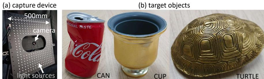
**Fig. 4.** Real-world experiment setup. (a): Our capture device has 256 LEDs on a printed circuit board ( $500 \times 500$  mm) at known positions. The CCD camera (FLIR Blackfly S;  $3072 \times 2048$  resolution) is fixed to the board at a known position by a 3D-printed frame. We put the target objects about 300 mm away from the device. (b): The three target objects used in our experiments: *CAN*, *CUP*, and *TURTLE*.
