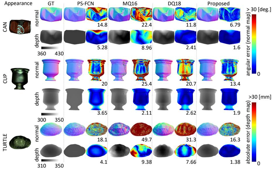
**Fig. 5.** Estimation results for our real-world dataset. For each scene and each method, we show the estimated surface normal map, the depth map, the normal error map, and the depth error map. “GT” shows the ground truth of normals and depth. The numbers underneath the error maps show mean angular error in degrees for the surface normal maps, and mean absolute error for the depth maps.
