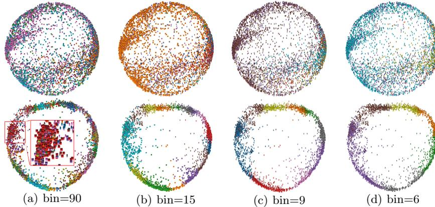
**Fig. 7.** Angular feature visualization of the 90-CSL-FPN detector on the DOTA dataset. First, we divide the entire angular range into several bins, and bins are different between columns. The two rows show two-dimensional feature visualizations of pulse and gaussian function, respectively. Each point represents a ROI of the test set with a index of the bin it belongs to.
