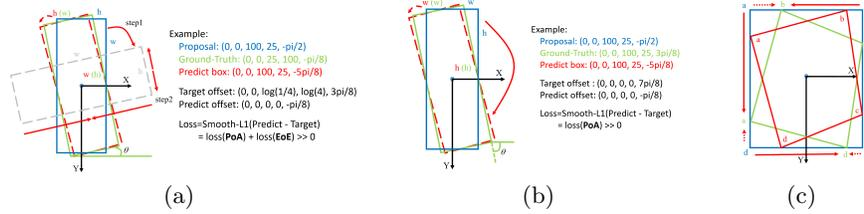
**Fig. 3.** The boundary problem of three categories of regression based methods. The red solid arrow indicates the actual regression process, and the red dotted arrow indicates the ideal regression process.
