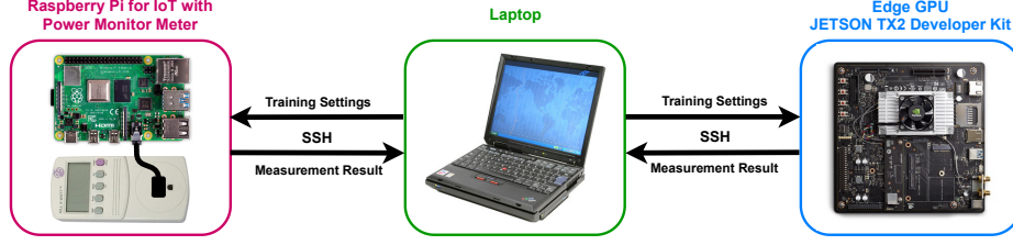
Fig. 4: The energy/running-time measurement setup with a laptop, a state-of-the-art Edge GPU [5] and a popular IoT device [8]
