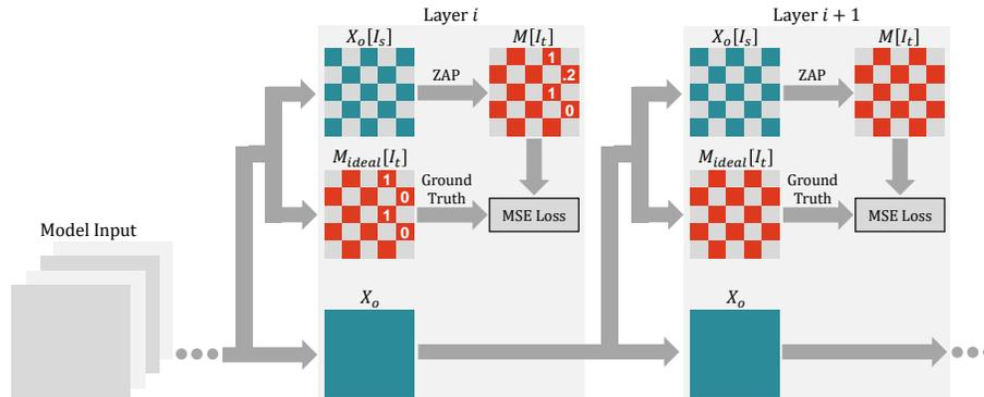
**Fig. 7.** Illustration of ZAP training. Each ZAP is trained independently in a teacher-student manner, enabling a parallel label-free training. The ground truth is the original layer ofm after a binary threshold operation ( $>0$ ). The CNN predictor is used with the ReLU activation function capped at 1.
