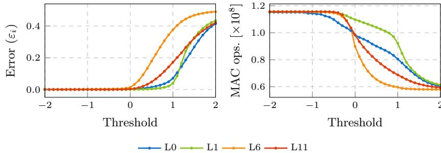
**Fig. 6.** ResNet-18 + ILSVRC-2012 example of different layers behavior in terms of error and MAC operations as a function of ZAP threshold.
