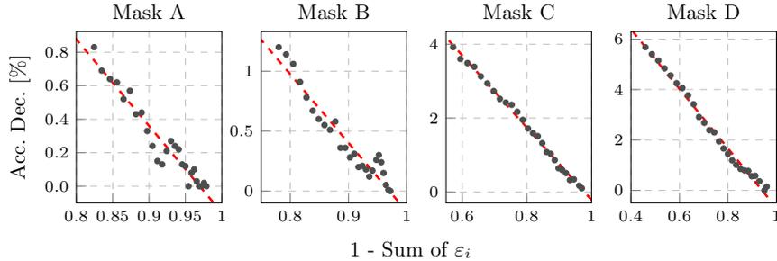
**Fig. 4.** AlexNet + CIFAR-100 top-1 accuracy decrease as a function of  $1 - \sum_{i=1}^L \varepsilon_i(\sigma)$ . Each dot represents a measurement with a different threshold: the leftmost and rightmost thresholds are 0 and 0.5, respectively. Measurements were taken in steps of 0.02.
