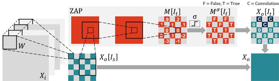
**Fig. 2.** Illustration of a single ofm channel convolution with ZAP.  $X_o[I_s]$  is computed based on a pre-defined pattern.  $X_o[I_s]$  is then subjected to ZAP, which produces a prediction map  $M[I_t]$ , followed by a thresholding step to form the binary prediction map  $M^\sigma[I_t]$ .  $X_o[I_t]$  is created according to  $M^\sigma[I_t]$  — a portion of the  $I_t$  ofm activations are predicted as zero-valued and skipped, whereas the rest are computed using Equation (1).
