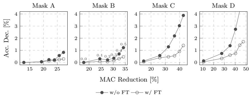
**Fig. 8.** Demonstrating the different operating points of AlexNet + CIFAR-100 with (w/) and without (w/o) fine-tuning (FT). Accuracy measurements are top-1. Threshold range is set between 0 to 0.5, in steps of 0.1. Each measurement corresponds to a threshold, as presented in “Mask B” plot.
