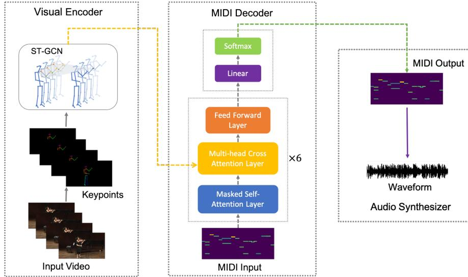
**Fig. 2. An overview of our model architecture.** It consists of three components: a visual encoder, a MIDI decoder, and an audio synthesizer. The visual encoder takes video frames to extract keypoint coordinates, use GCN to capture the body dynamic and produce a latent representation over time. The MIDI decoder take the video sequence representation to generate a sequence of MIDI event. Finally the MIDI event is converted to the waveform with a standard audio synthesizer.
