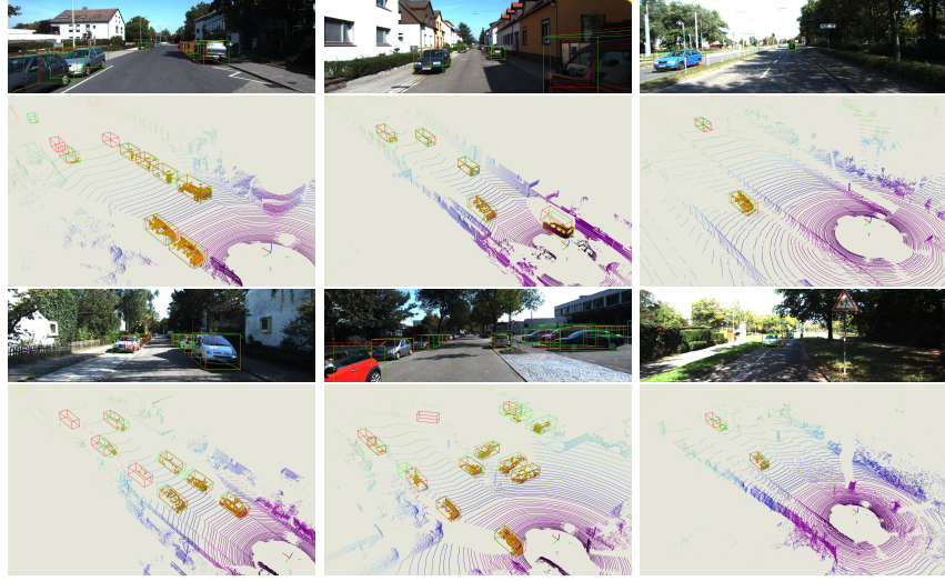
Fig. 5. Qualitative results on KITTI validation set. Red boxes represent our predictions, and green boxes come from ground truth. LiDAR signals are only used for visualization. Best viewed in color with zoom in.
