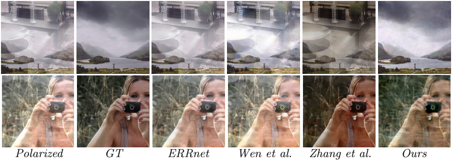
Fig. 3: Visual comparison for synthetic polarized dataset. From left to right are: polarized images ( Polarized ), transmitted scene ( GT ), ERRnet [19], Wen et al. [18], Zhang et al. [4], and our transmitted results ( Ours ), respectively.
